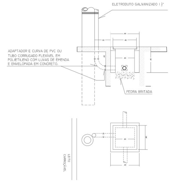
**DETALHE CAIXA PASSAGEM SEM ESCALA**
